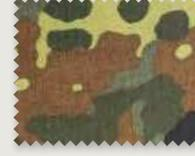
**110DTEX PA6.6 SILICON** (100% polyamide). Lightweight, double-sided silicone-coated and printed Nylon fabric in 5-color camouflage. The material according to TL 8305-0278 is used for rain covers.
