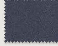
**T-Vent 3L** (Outer layer: 92% polyamide, 8% elastane, inner layer: 100% polyamide, membrane: 100% polyurethane). This robust, elastic, wind- and waterproof 3-layered material is used for high-quality hardshell jackets. This ultrathin non-porous membrane is extremely waterproof and offers a high air permeability and stretchability.
